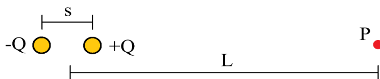
Figure 2. The figure given on the activity. The two circles ('+Q' and '-Q') are the equal magnitude, oppositely signed charges that constitute the dipole. L is distance from the dipole's midpoint to the observation point P and s is the distance between charges in the dipole. Students were to work in the regime where L \gg s .
